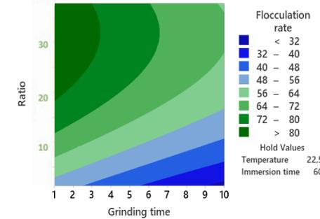
Fig. 1. Contour plot - flocculation rate and equation.
