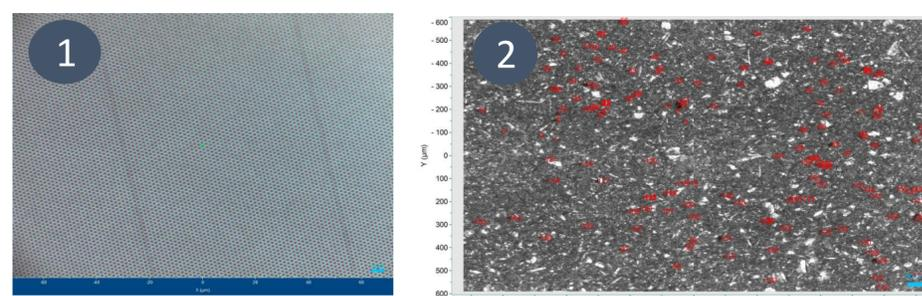
Figure 3 – Silicon wafer filter surface before (1) and after (2) filtration.
