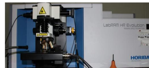
Figure 2 – Raman Microscope
