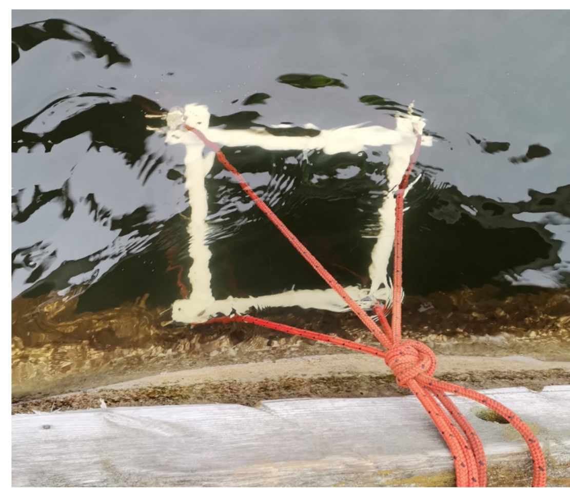
Figure 1: Experimental setup with PET sheets on a frame placed in a river
