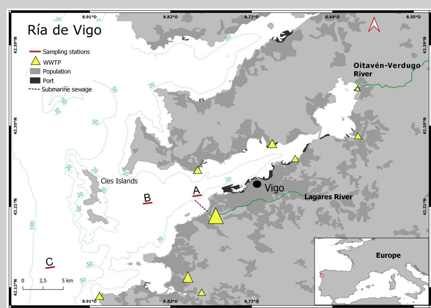
Surface water samples using manta trawl nets (mesh size 330 µm) were taken monthly at three stations for one year during the Vigo Radial cruise for a total of 32 samples. The manta was towed for 10 min at a vessel speed of ~3 knots. Samples were washed using filtered seawater (0.200 mm) and then transferred to amber glass bottles and frozen at -20 °C until analysis.
