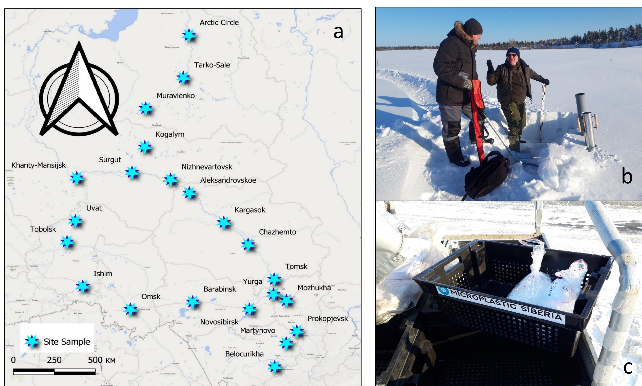
Fig. 1. Map of the sampling locations (QGIS 3.18.3) (a), conducting snow core sampling (b) and packaged samples (c).
