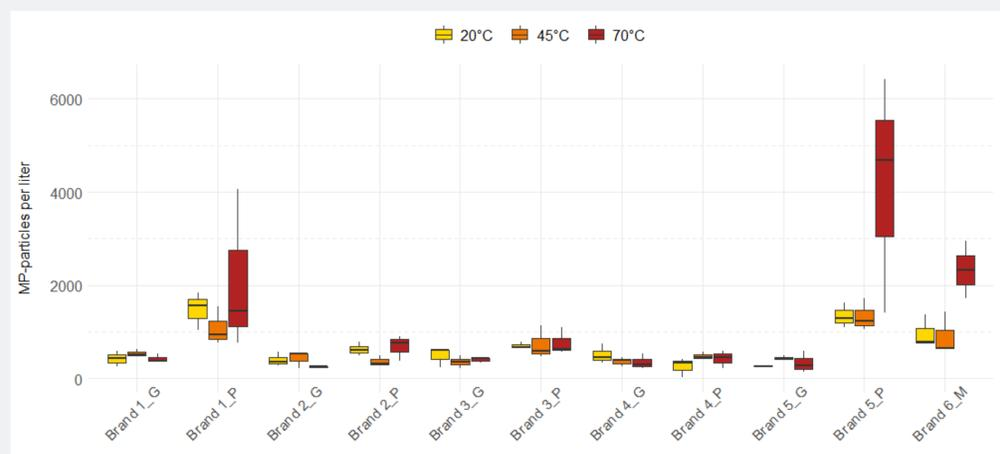
Fig. 2: Microplastic release from different preparation temperatures.
