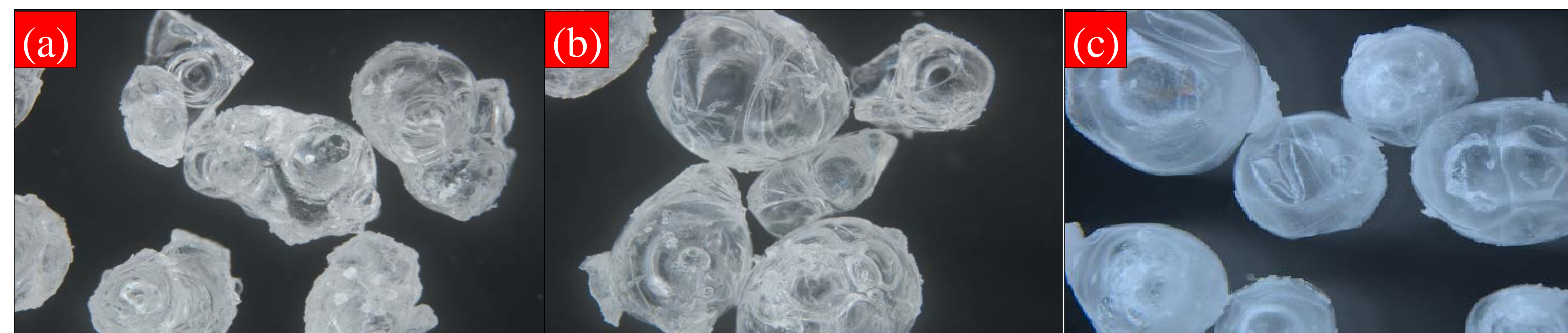
Figure 2. Microplastics swollen and pitted after 48-hour, 90°C digestions with (a) KOH, (b) NaOH and (c) H 2 O 2 at 2.5X magnification
