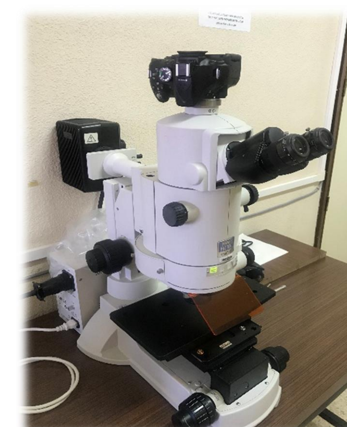
Visual counting and classification in a stereomicroscope
