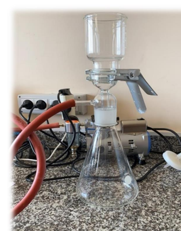
Vacuum assisted filtration and washing with Milli-Q water
