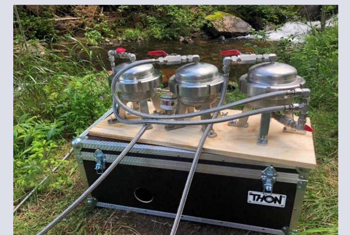
Custom-built filtration device (AAU UFO-system) with one 300 μm filter followed by two 10 μm filters installed
