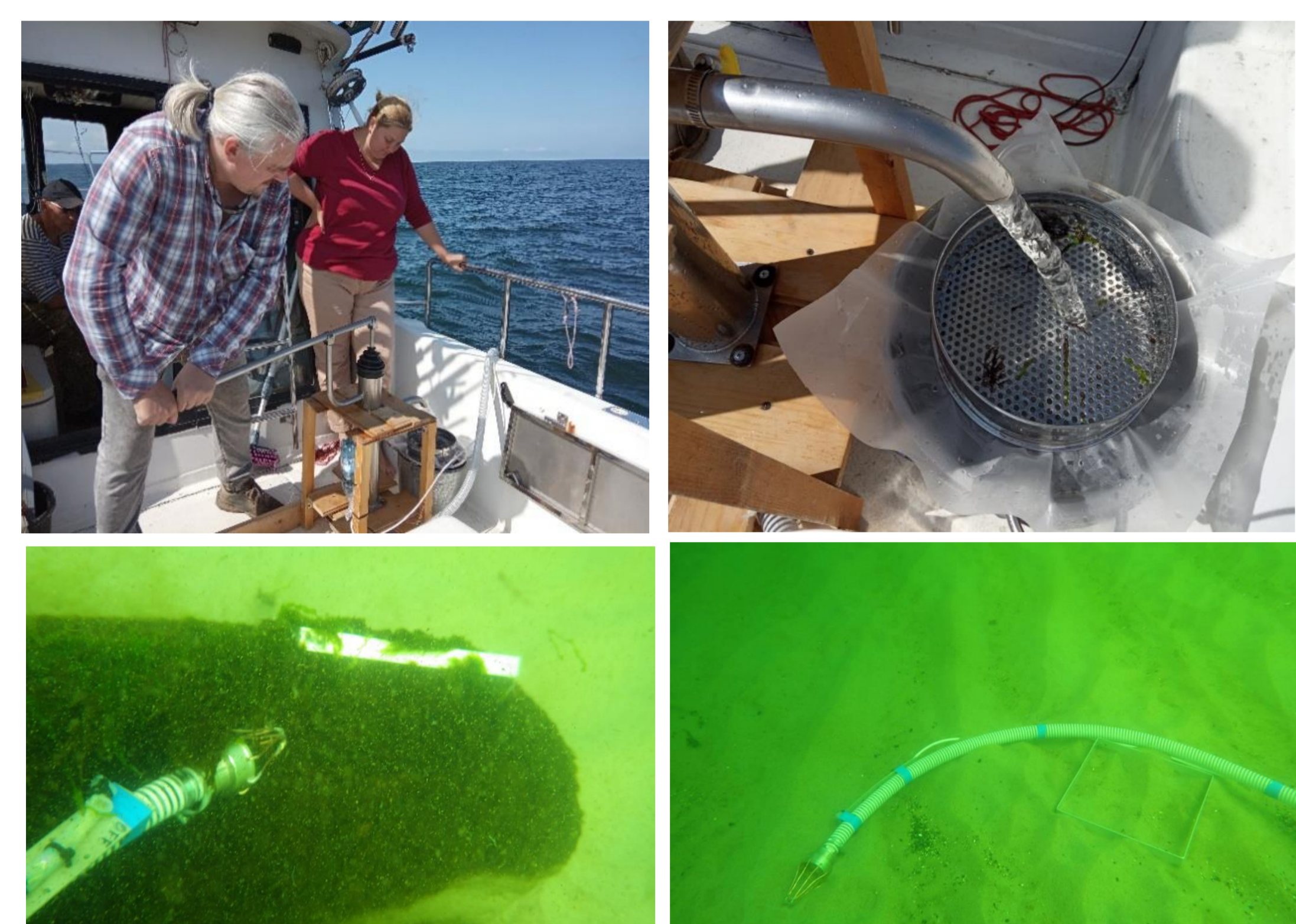
Fig. 3. Sampling of macrophytes was performed: (a) directly on underwater slope from growing thickets and algae-free water in surroundings (hand pump was used); (b) by the diver working from the boat, in shallow coastal waters (areas with filamentous algae (at depths of 3.2 and 4 m) and with perennial algae Furcellaria (depths of 5.6 and 8.2 m).
