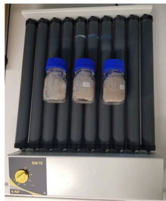
Figure 1: Mixer with glass bottles filled with sand, water and polymer pellets to test the fragmentation.
