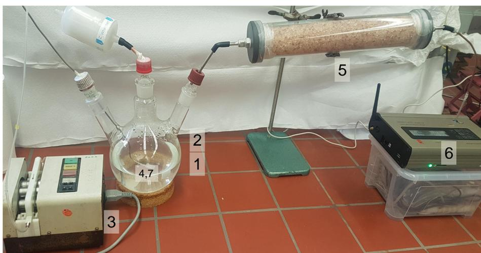
Fig. 2: Experimental setup for the bubble bursting experiments with MPP. The numbers are explained in the description above.
