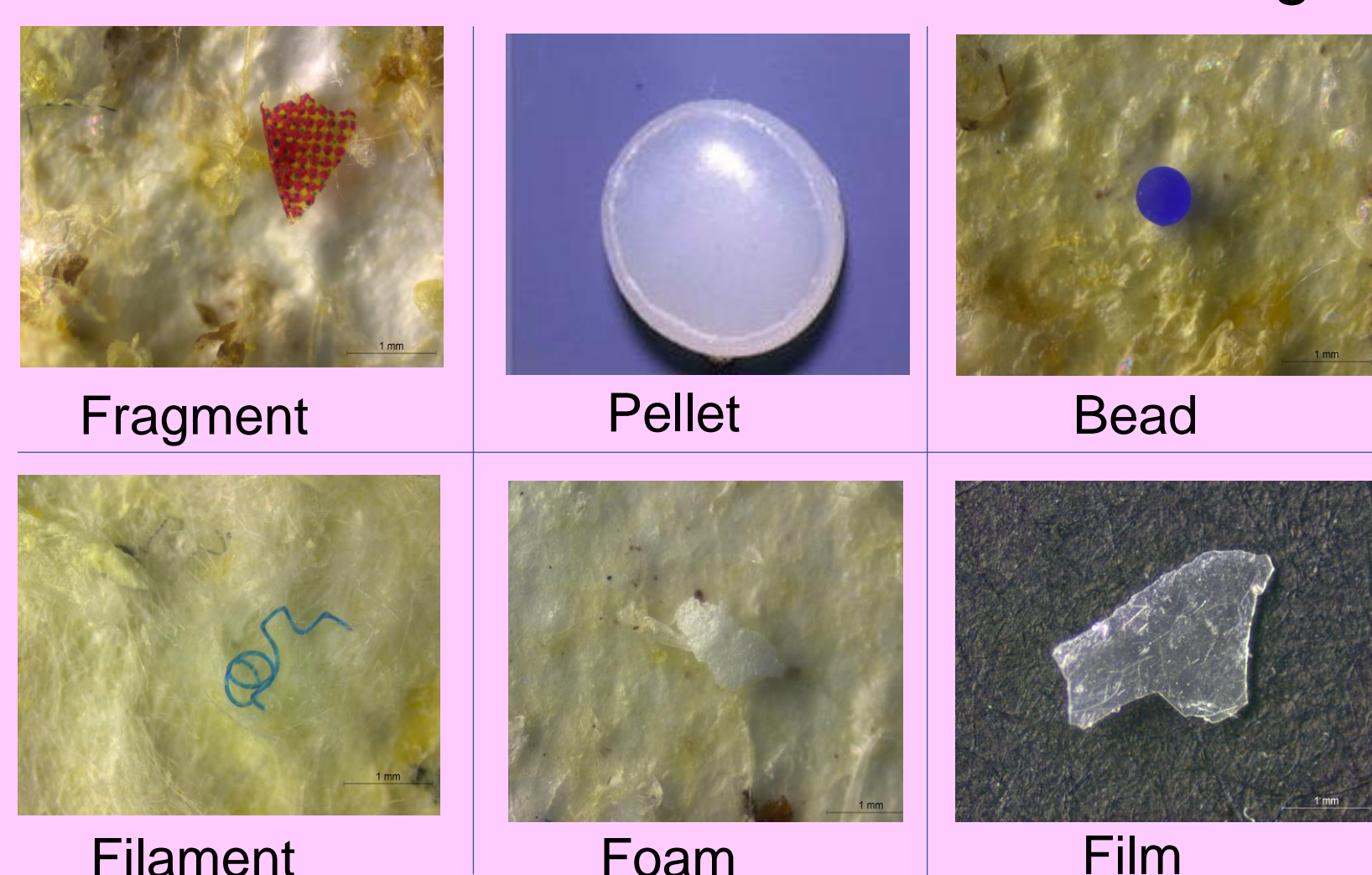
Figure 2. Types of particles found in samples – plastic fragments, pellets, beads, filaments, foams, films.
