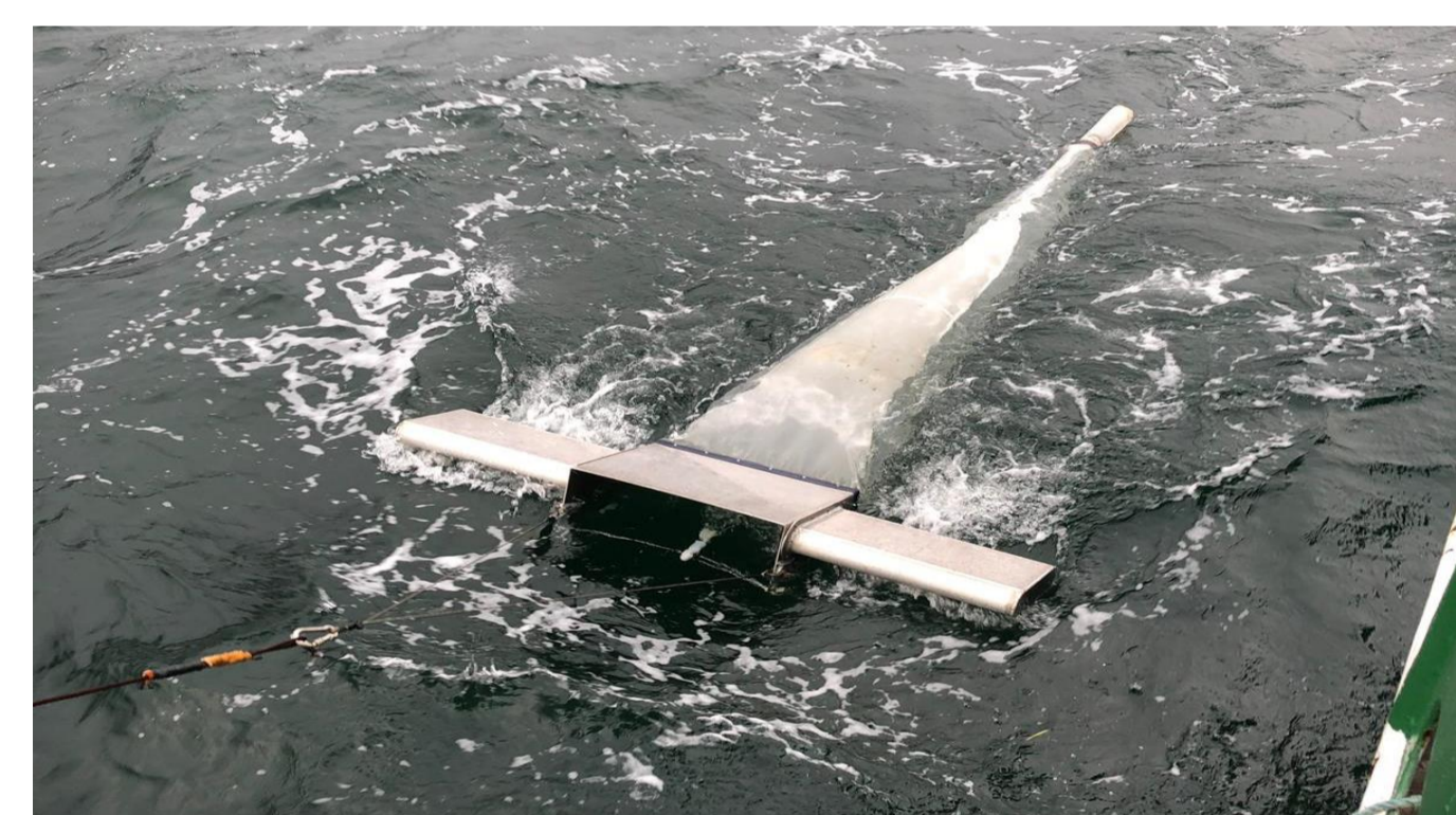
Figure 3. Manta trawl used for sampling
