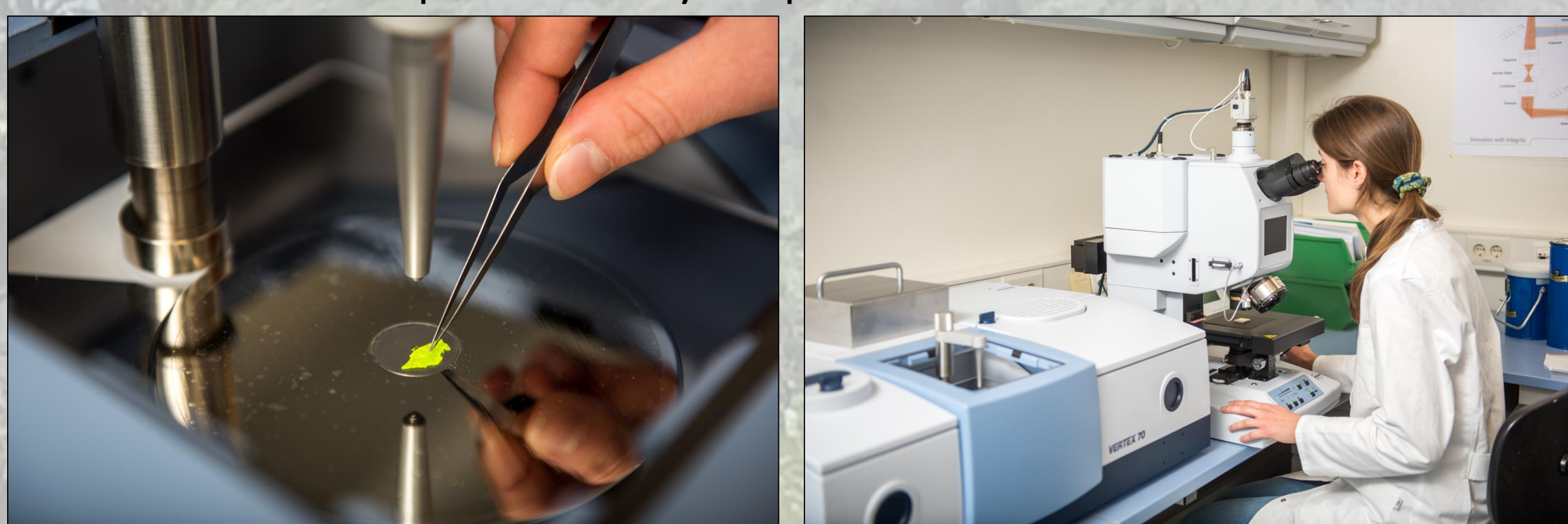
Fig. 2 Sonja M. Ehlers identifying polymer types using FTIR (Vertex 70, Bruker, Ettlingen, Germany) at the Federal Institute of Hydrology in Koblenz, Germany.
