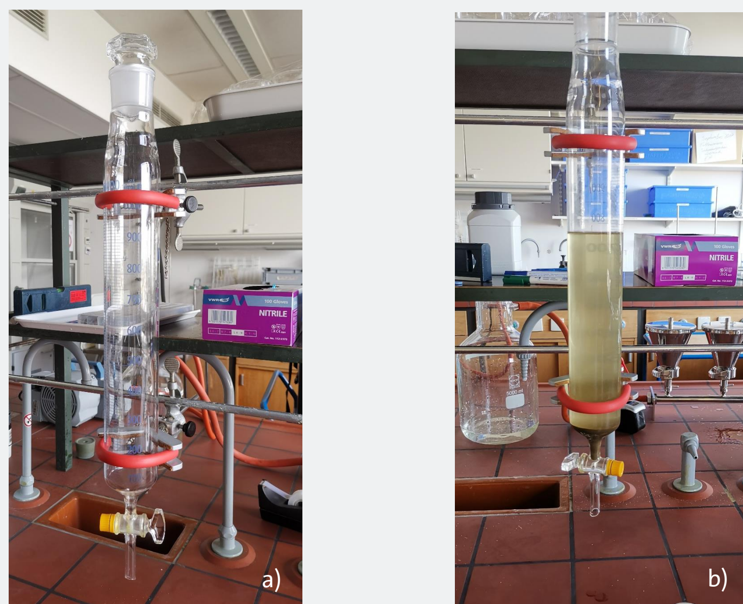
Fig. 2: Density separation glass column when a) empty b) filled with NaI and sample material.
