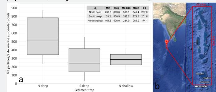
Fig. 6: a: Distribution of MP particle concentrations in MP particles g<sup>-1</sup> dw mss per sediment trap with descriptive statistics. b: Theoretical rectangular sea area (835 x 163 km<sup>2</sup>) around the Maldives to illustrate the extrapolated and simplified results of about 860 kg MP < 1 mm which sediment every day in this area.
