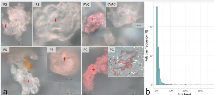
Fig. 4: a: Selection of PS, PC, PVC and EVAC polymer images taken with  $\mu$ Raman-spectroscopy. b: Size distribution of all counted microplastic particles as relative frequencies (%) according to their major dimension (bar width of 40  $\mu$ m).
