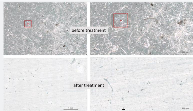
Fig. 2:  $\mu$ Raman-spectroscopy mosaic images of a preliminary test sample before (images above) and after (images below) treatment with 85% H<sub>3</sub>PO<sub>4</sub>. Chitin-sickle structures are no longer visible after the treatment.
